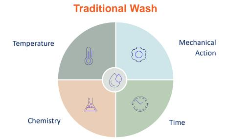
Washing processes rely on temperature, chemistry (detergent) and cycle length.
